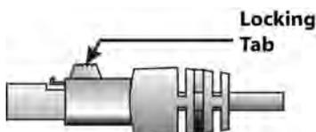
When disconnecting a power source from the SprintPack Power Manager or LTV<sup>®</sup> Ventilator, always depress the locking tab on the power pigtail connectors.
