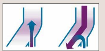
Expiration: Gas flow flipped away from the nasal prongs to the expiratory tube. The residual gas pressure provided by the continuous gas flow creates a stable CPAP throughout the respiratory cycle.
