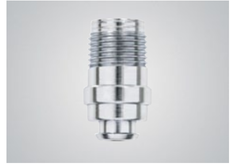
03837 Connector, tailpiece Oxygen, 7/16-27
