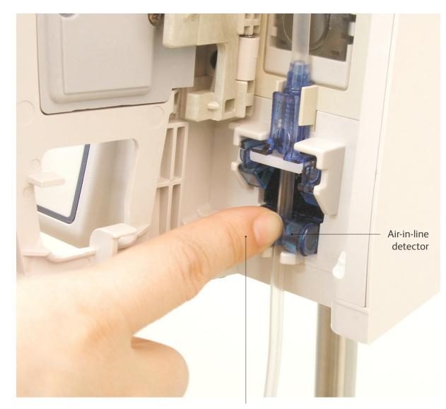
Use a fingertip to firmly push the tubing toward the back of the air-in-line detector.
